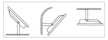
Install the LED flood lights in the ground, wall, and ceiling
