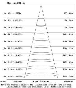
when the luminaire is at different distance.
